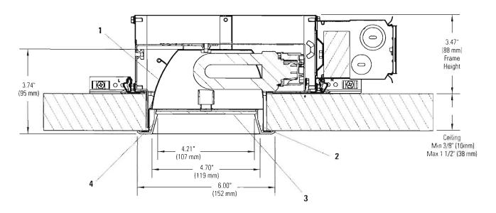
Complete Fixture consists of Frame-In Kit and Reflector Trim. Select each separately.
